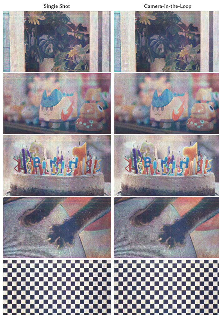
Fig. S2. Active camera-in-the-Loop (CiTL) reduces noise and improves color fidelity. The first column of this image depicts experimentally captured color holograms. The second columns shows images that were iteratively improved with a camera in the system using the active CiTL algorithm of Peng et al. [2020].
