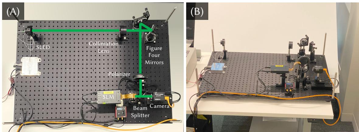
Figure 9: Experimental setup A top view of our system with labeled components and an approximate beam path drawn in green is depicted in (A). A side-view of the system is provided by (B). Note that the hologram is formed directly on the bare camera sensor with no lens or eyepiece between. This configuration allows us to validate our method, but for a human-viewable system, an eyepiece must be added between the hologram plane and the user's eye.
