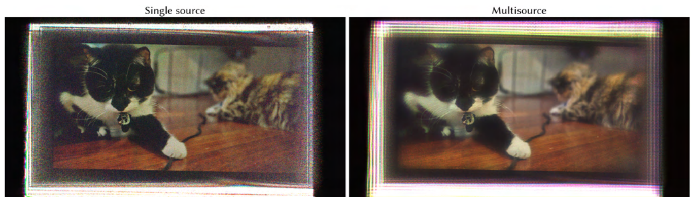
Fig. S13. Raw Camera Capture : We show examples for both single source and multisource of the raw camera images before any alignment or cropping is applied. The only processing is combining the three monochrome captures into a color image.
