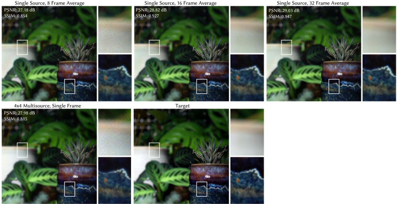
Fig. S7. Temporal Multiplexing with More Frames: In simulation, we compare multisource holography with 16 sources to temporal multiplexing with 8, 16, and 32 frames. Multisource holography performs similarly to temporal multiplexing with 8 frames: even though there are more incoherent averages in our approach, multisource holography has fewer degrees of freedom compared to temporal multiplexing, which limits the amount of despeckling. As the number of frames increase, temporal multiplexing outperforms multisource, but at the expense of temporal bandwidth.
